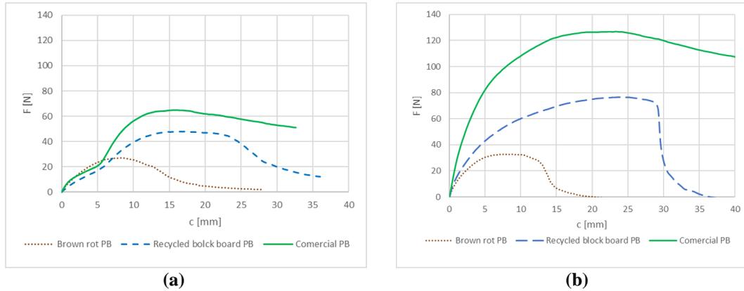
**Fig. 3 Force-displacement diagram of stress loading in the angular plane – average value (a) wooden dowel joint, (b) confirmat joint.**
