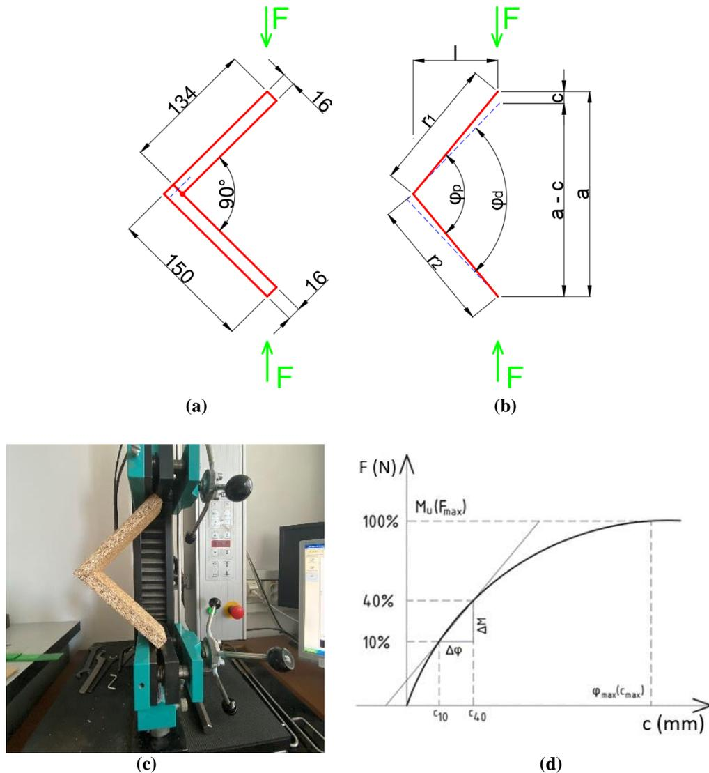
**Fig. 1 Specimen for stiffness and load capacity (a) dimensions of the specimens, (b) loading scheme with geometrical characteristics (c) execution of the test and (d) force deformation diagram.**
