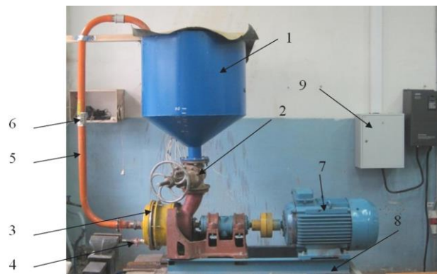
Fig. 1 The general arrangement of the test bench: 1: tank; 2: gate valve; 3: hydrodynamic homogenizer; 4: drain ball valve; 5: circulation pipe; 6: ball valve; 7: motor; 8: support frame; 9: control panel.
