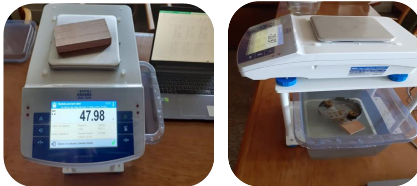
Fig. 2 Measurement of the density of beech wood samples.
