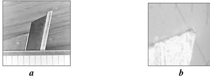
**Fig. 5 Measurement of the radius of rounding of the blades of the milling cutter knives *a* – the knife of the milling cutter; *b* – the top of the experimental knife of the milling cutter under the microscope.**
