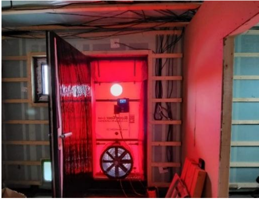
Figure 1. Blower-door test: Example of the measuring device installed in the door frame.
