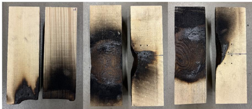
Fig. 7 Photo documentation of samples after scrapped of the charred layer (0°, 90°, 45°).
