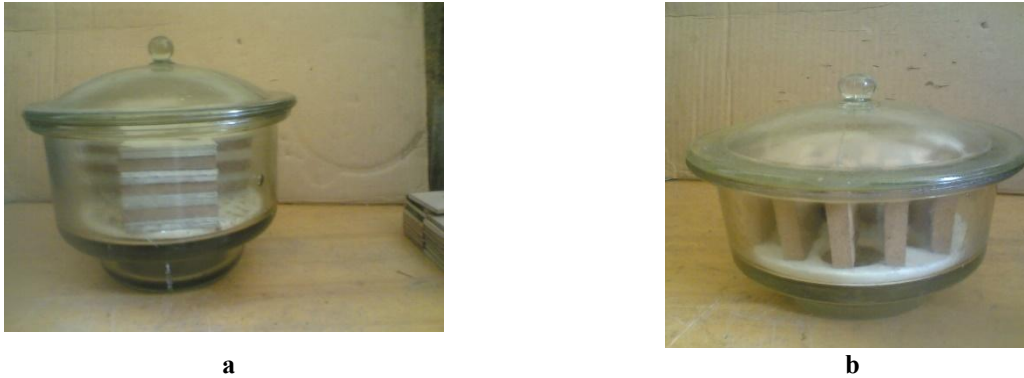
Fig. 1 Location of the samples: a - samples in hygroscopic covers placed in a water-charged desiccator; b - samples in a sulfuric acid-charged desiccator.
