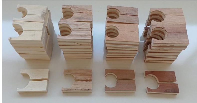
Fig. 3 Post-test images of splitting strength test samples (from left to right: Groups 1-4).
