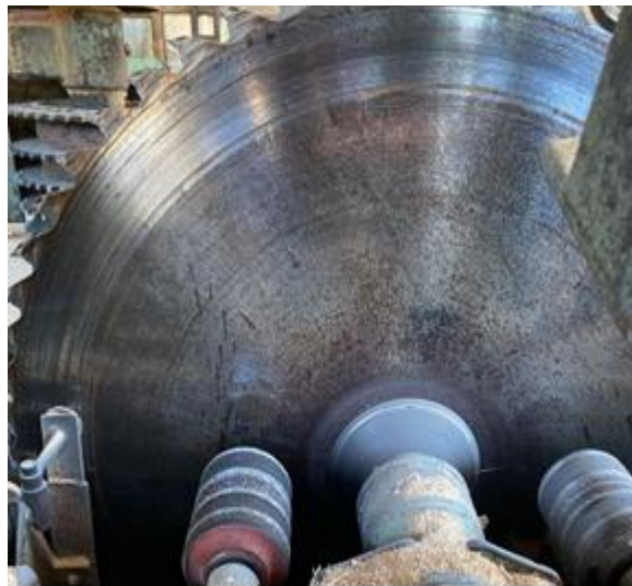
Fig. 2 Circular saw blade D = 1060 mm.
