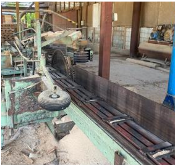
Fig. 1 Circular saw mill Kara KallionKonepaja Oy – Finland, general view.
