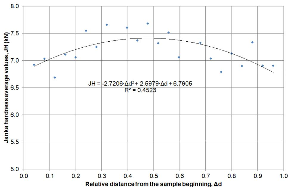
**Fig. 2** Janka hardness average values for the combined air drying process of beech samples in a function of relative distances from the sample beginning.
