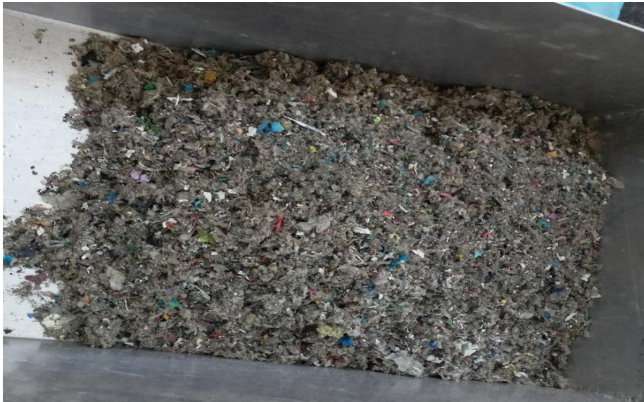
Fig. 1 Ground recycled iRDF waste prepared for its mixing with wood particles and adhesive mixture for the particleboard production.
