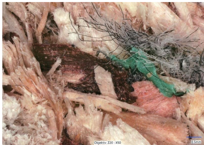
Fig. 3 Microscopic structure of the core layer of modified particleboard with the presence of recycled iRDF waste.
