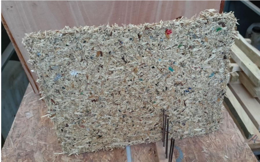
Fig. 4 Recycled iRDF together with wood particles present on the surface of pressed single-layer particleboard.
