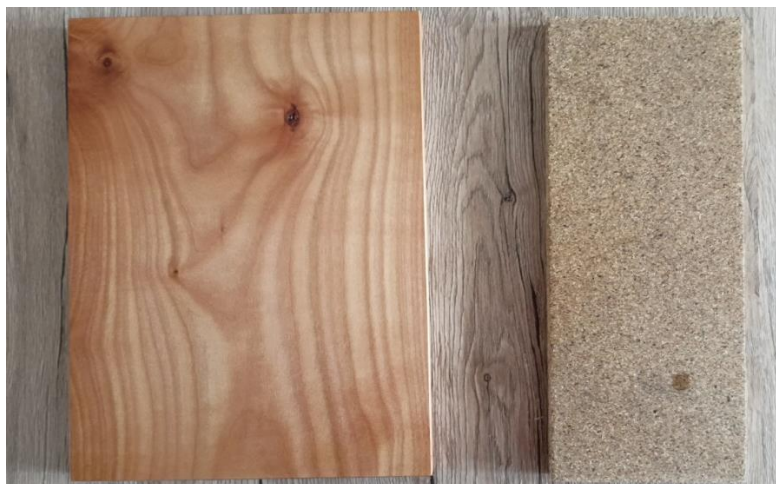
Fig. 5 Modified three-layer particleboard with the presence of 15% iRDF in the core layer surface treated with veneering for demonstration purposes (left) and raw particleboard with the presence of 15% iRDF in the middle layer without surface treatment (right).
