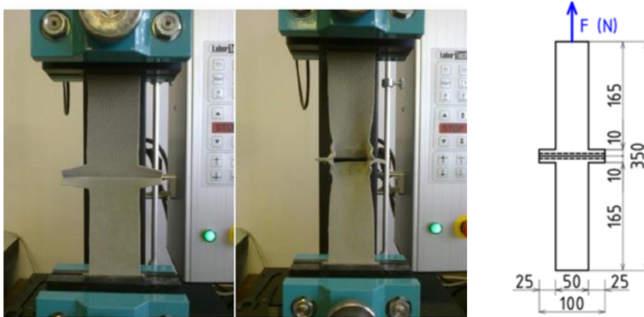
Fig. 3 The loading scheme and sample dimension.
